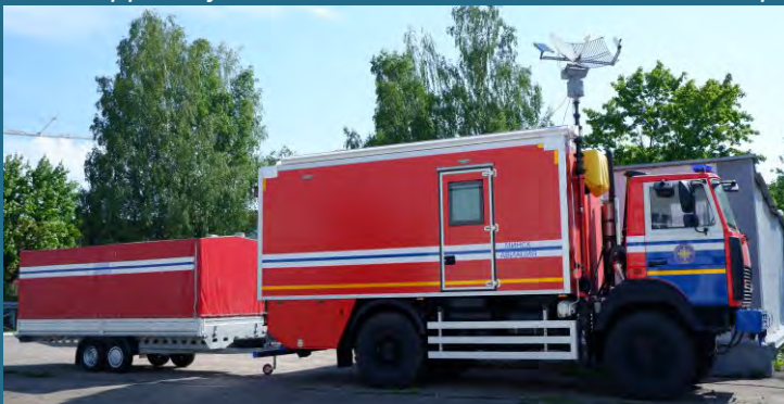
GCS based on a MAZ type vehicle with a body superstructure, a life support system for the crew and a trailer for transporting UAVs
